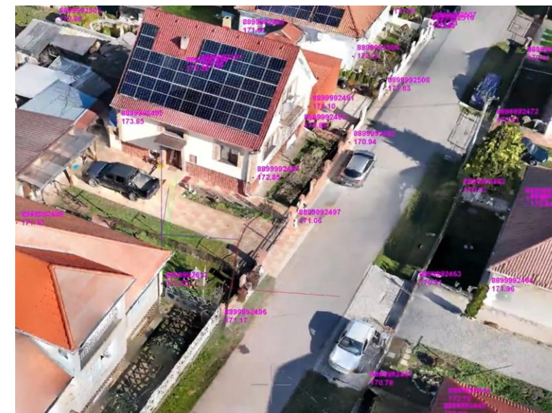
Example of identification, evaluation and determination of point coordinates in the national coordinate system
