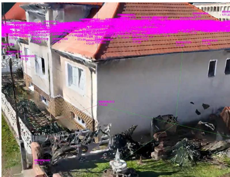
Example of identification, evaluation and determination of point coordinates in the national coordinate system
